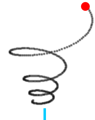
ion's Larmor motion around radial B-field
